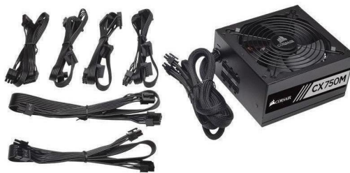
Example of a semi modular PSU and some removable cables
